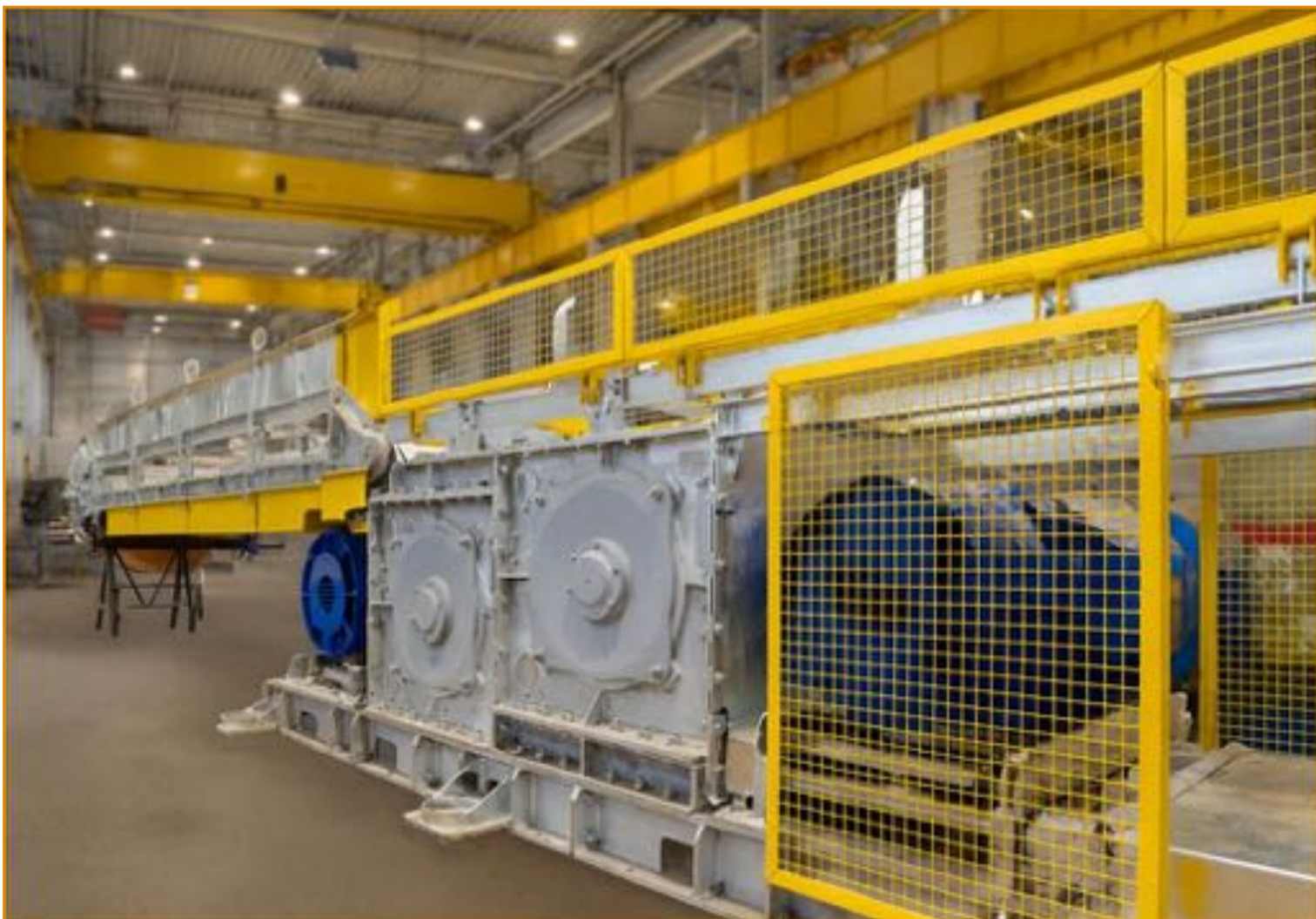
Fig. 1 AR-Project 1000 Belt Conveyor, length 150m, designed for hauling mined material.
