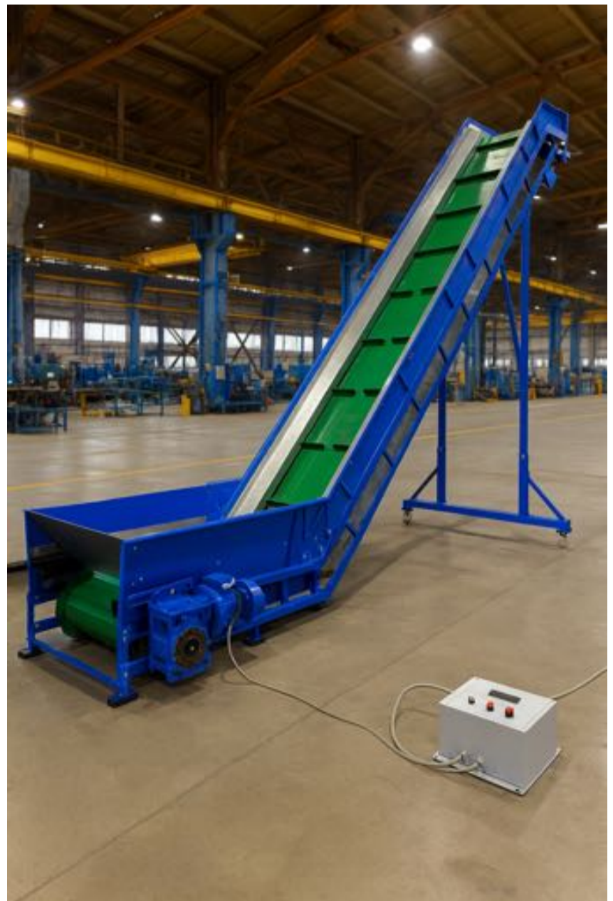
Fig. 8 Mobile conveyor for recycling sector (bottles) - one of the realised projects.
