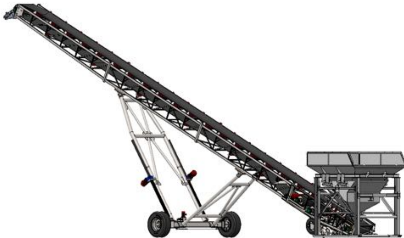
Fig. 6 Mobile conveyor in operating configuration and working position
