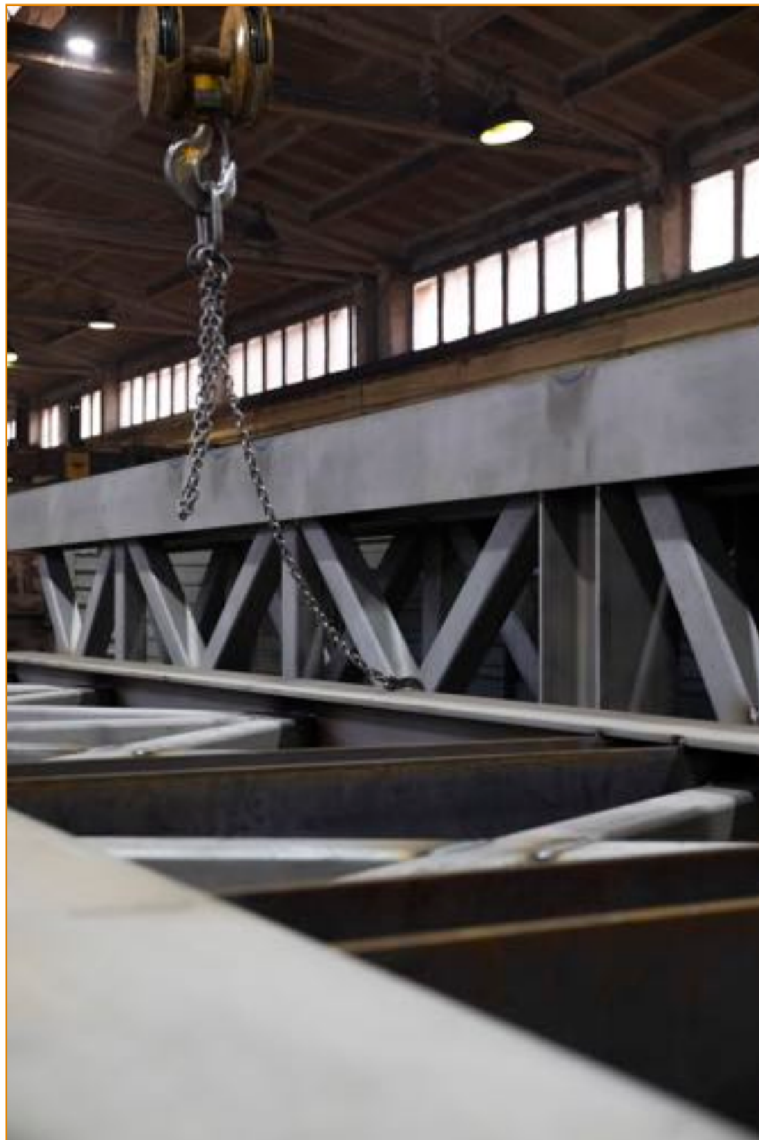
Fig. 1 Fabrication of structural components for the mounting and integration of feeders and vibrating screens.
